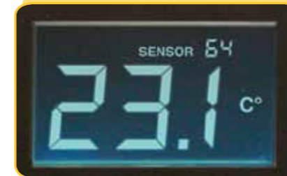
LCD display for at-the-rack monitoring of all sensor data
