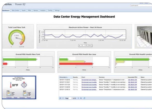
Data center power management software gathers data from sensors and iPDUs and displays information on a single, organized dashboard.
